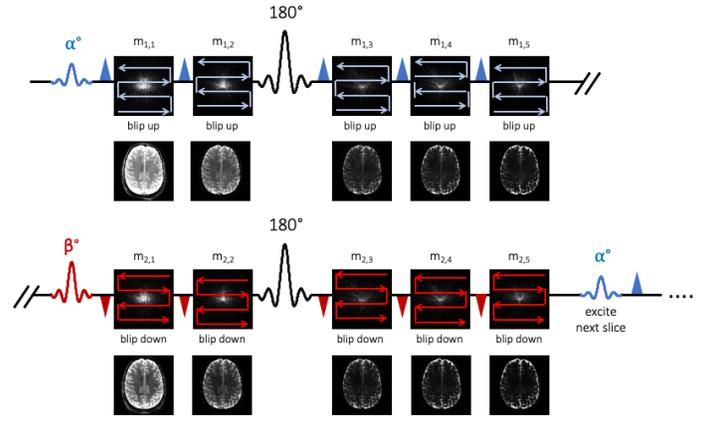
Figure 1. The sequence diagram of VUDU-SAGE
