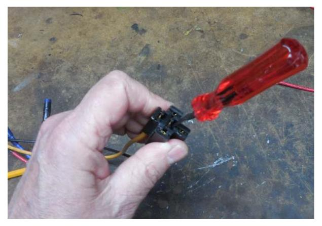
Put the tool in from the front (relay) side, push on the tab and out it comes.
