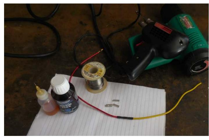
These joints are nice and slender and usually you can get them back into the loom just like they were before. The tubing also grips the wire (adhesive!), is waterproof (adhesive!) and sort of rigid-like when it cools. A really solid joint, electrically and mechanically.
