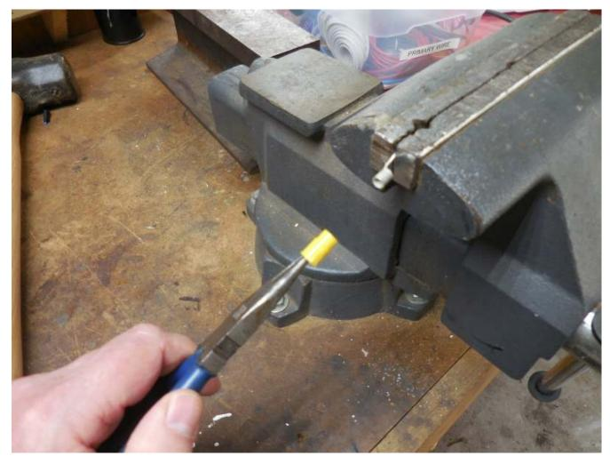
Connectors where the insulation covers the metal like butt connectors or the female side of bullet connectors are harder - I alternately score the plastic with my utility knife and peel at the plastic with my pliers till it comes off.
