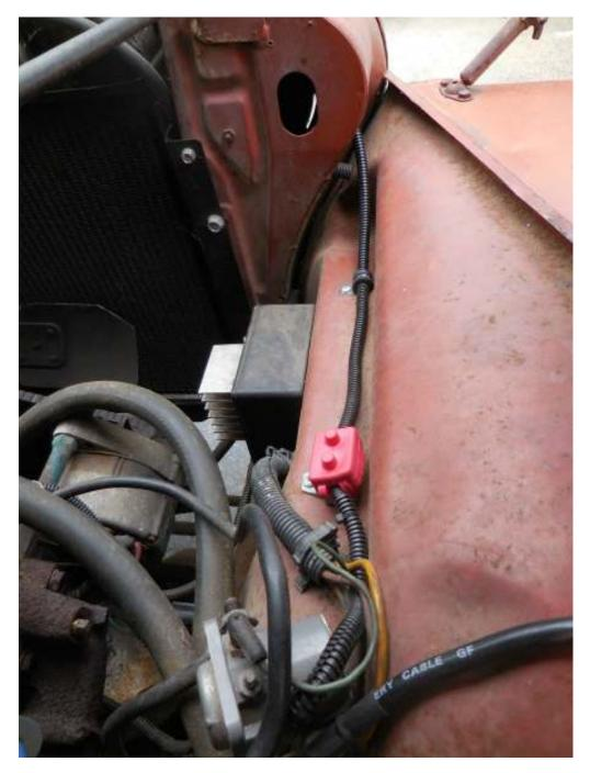
You can see one wire clamp and the loom disappearing into an existing hole in the grille. The wire and loom go across the underside of the grille (behind and above the grille bars), supported by the existing loom that contains the factory lighting wiring.
