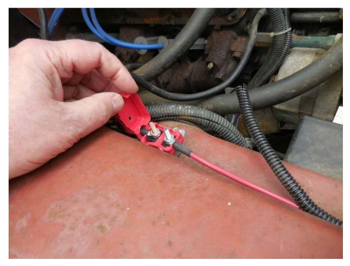
This is the battery side, showing the BlueSeas circuit breaker and its rubbery cover. I suspect this is the WVE circuit breaker you can buy from RockAuto inexpensively. The rubbery cover is available on Amazon. Not much to see here.
