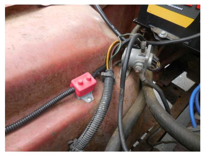
This is the opposite side. You can see that the big fat wire is protected here by loom, from the solenoid, to the circuit breaker, and across the fender. Another view -
